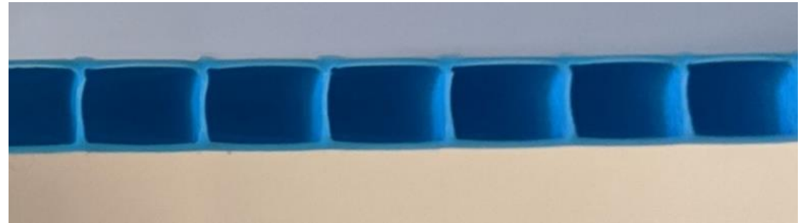
Figures showing the ribs in between the sheets of plastic. The plastic is strongest when these ribs are parallel to the loading axis
